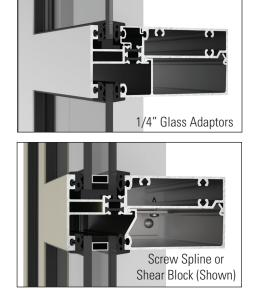
This system utilizes dual 6/6 polyamide iso struts that secures the inner and outer mullion pieces together. This strut provides a thermal barrier that saves energy and limits heat transferance. It will not degrade, break due to the glass-fiber reinforcement. This also allows for dual-finish capability.
